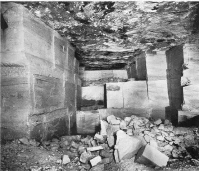
The size of the blocks removed is clearly seen in this working face. It would appear work stopped here at the end of the day and never restarted. This was, perhaps, one of the last faces to be worked in 1960. Photo Nick Catford
